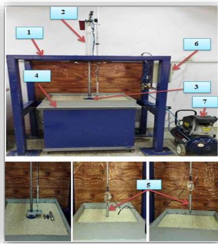
**Figure 2. General view of the manufactured apparatus (1-Steel loading frame, 2- Axial loading system, 3- Model footing, 4- Steel container, 5- Strength measuring device, 6- Control system, and 7- Air compressor system).**
