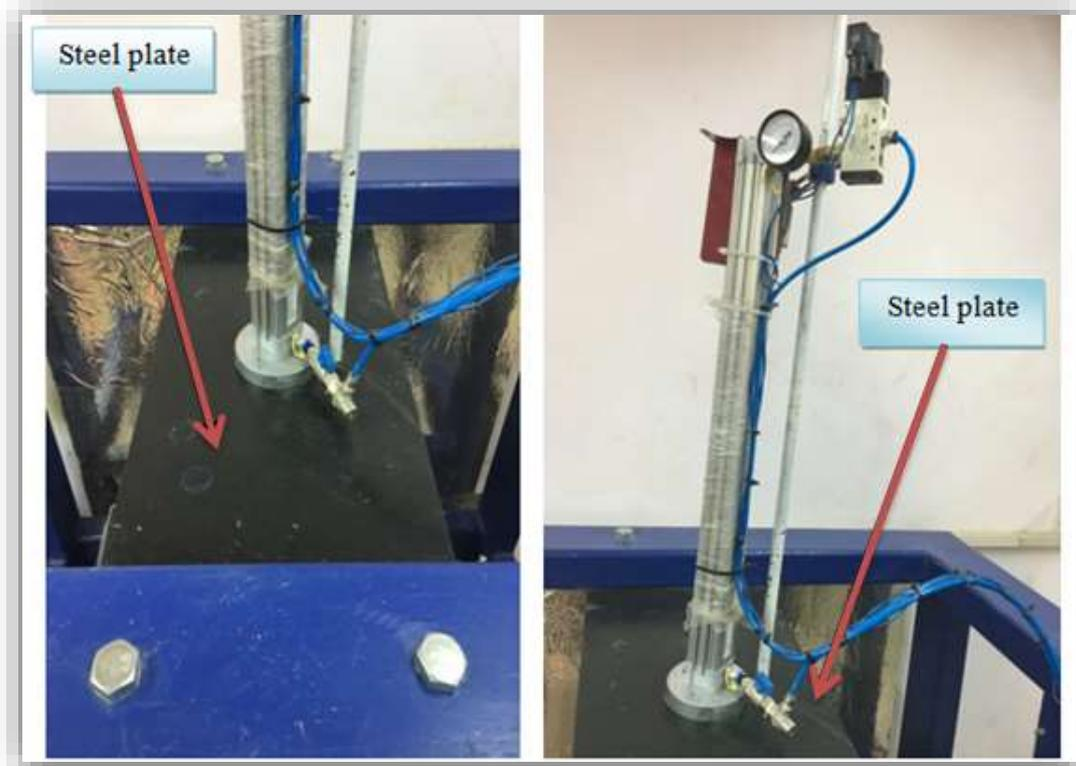
Figure 3. Steel plate to support the jack.
