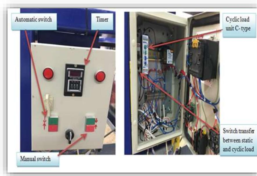
Figure 4. Control system – a general view.
