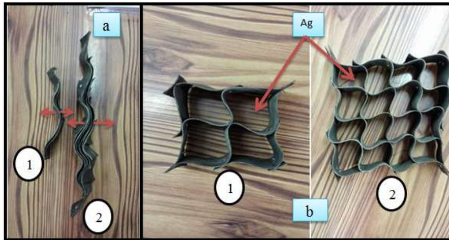
**Figure1.** Geocell used. (a) geocell before expanding. (b) top view of the geocell mattress after expanding. (1) geocell mat of width  $b_1=100$  mm. (2) geocell mat of width  $b_2=200$  mm.
